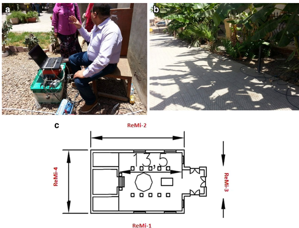
Fig. 6 a, b Samples of ReMi profile conducted inside and around Ben Ezra Synagogue
