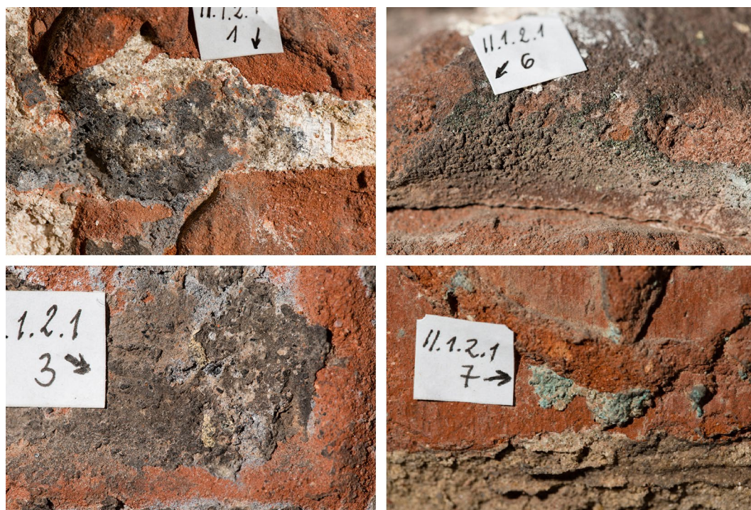
Fig. 3 Green and grey patches of color on the ceramic tiles and grey patches on mortar joints. Sampling sites. Photograph by D. Kwiecień
