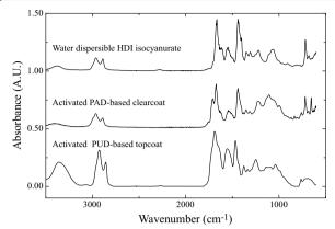
**Fig. 4** FTIR spectra of two 2KWBPU coatings activated with water dispersible HDI isocyanurates, developed for conserving OPS by Calder; white topcoat (N9688A) from NCP using PU dispersion (PUD) as co-reactant and clear coat using polyacrylic dispersion (PAD) as co-reactant (Bayhydrol 2542, Bayer)
