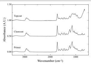
**Fig. 5** FTIR spectra of 1KWBPU systems; Imron 1.2 HG-C clearcoat, Imron 1.5 Pr grey primer and Imron 1.5 ST-D direct-to-metal white topcoat. The three spectra all display a single band in the 1730–1650 cm<sup>-1</sup> region
