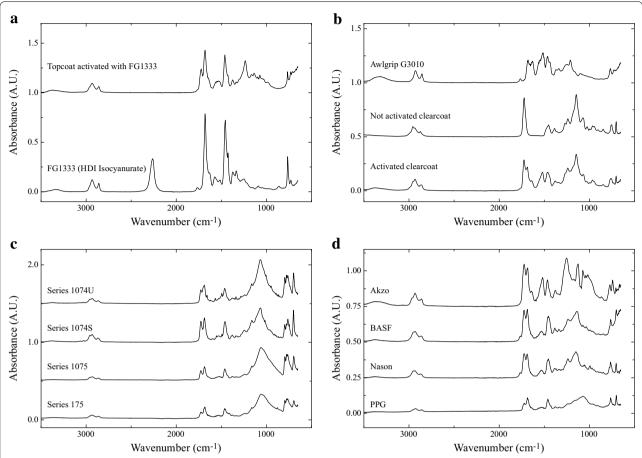
Fig. 3 FTIR spectra of various 2KSBPU samples: a Imron FG1333 and Imron 2.1 white topcoat activated with FG1333; **b** Awlgrip G3010 convertor, Aircraft 2000 clearcoat unactivated and activated with G3010; **c** *black, red, orange* and *yellow* EnduraShield topcoats from the 175, 1074U, 1075 and 73 Series; **d** Akzo Nobel (Akzo 683-3-7 clear), PPG (Deltron DBU *blue*), Nason (FullBase 3.5 VOC *red*) and BASF (Glasurit 22 *blue*)
