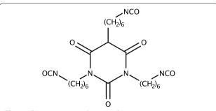
**Fig. 1** HDI isocyanurate indicates a HDI trimer containing an isocyanurate ring
