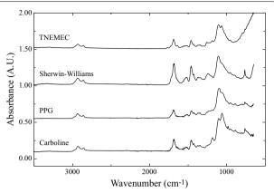
**Fig. 6** FTIR spectra of four black 2KFPU topcoats from different manufacturers; Fluoranar Series 1072 by Tnemec, Fluorokem by Sherwin-Williams, Coraflon by PPG and Carboxane 950 by Carboline. All of them exhibit a strong IR double absorption at ca. 1110 and ca. 1065 cm<sup>-1</sup> in accordance with the typical F–C stretching region
