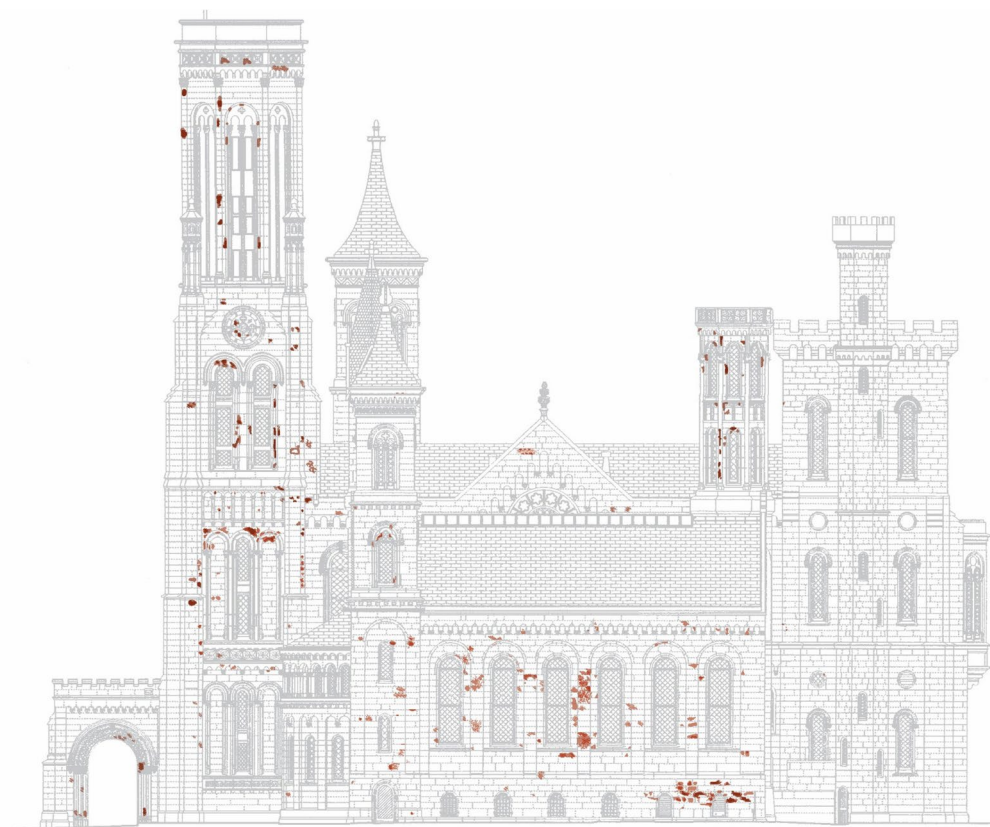
Fig. 4 West architectural elevation of the Castle showing rock varnish. An estimate of the areal distribution of Mn-bearing rock varnish on the building in 2015 is represented by red-brown patches
