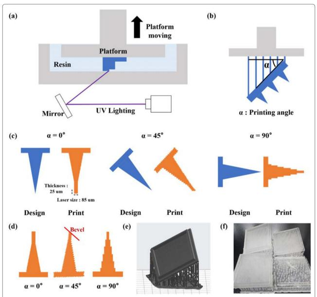
Fig. 1 a The schematic diagram of SLA 3D printing. b The schematic diagram of 3D printing angle setting. c-d The schematic diagrams of original design and printed microneedles according to printing angles. e An image of 3D printing setting at the angle of 45°. f Printed molds (0–30°)
