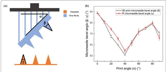
Fig. 4 a The schematic diagram of 3D printed microneedle and PI microneedle. **b** The bevel angle of the microneedle according to the print angle. (α: printing angle,  $\beta$ : 3D printed microneedle bevel angle,  $\gamma$ : PI microneedle bevel angle) (n = 10)
