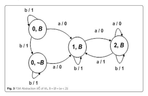
transition (0, a, (w > 2), 0, up, 1), where up contains w := 1. Correspondingly, the abstraction FSM moves to state 1 producing the output 0. Thus, in the abstraction FSM we have the transition ((0,  $\sim B$ ), a, 0, (1, B)).
