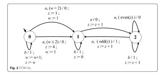
FSM we have the transition  $((0, \sim B), b, 0, (0, \sim B))$ . Furthermore, any value of  $w \ge 2$ , which also satisfies  $\sim B$ , executing the outgoing transition from state 0 of  $M_2$  under b updates the value of w in such a way that  $\sim B$  still holds. Thus, for all these configurations with  $w \ge 2$ , in the abstraction FSM we have the transition  $((0, \sim B), b, 0, (0, \sim B))$ .
