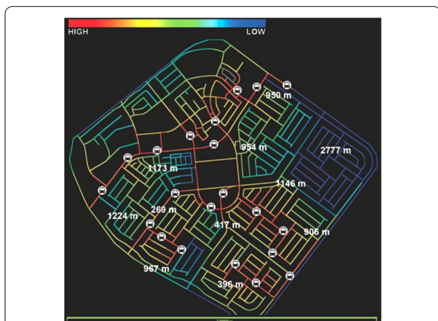
Fig. 11 Bus-Stops distances to residents in the whole Al Barsha North District, calculated by the DepthmapX tool
