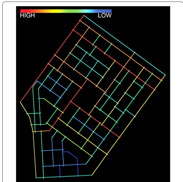
Fig. 29 More spatial integration of mobility networks after the inclusion of redeveloped walkways/cycling lanes, as simulated by the DepthmapX tool
