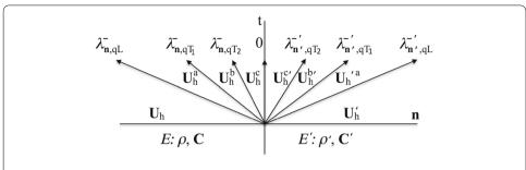
Fig. 1 Sketch illustrating the Rankine–Hugoniot jump conditions in the Riemann problem in the 3D case
