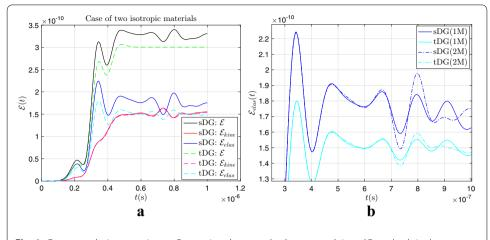
**Fig. 6** Energy evolution over time. **a** Comparison between both space and time dG methods in the heterogeneous isotropic case; **b** comparison between homogenous and heterogeneous isotropic cases
