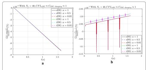
**Fig. 2** Decreasing of the total energy over time by both space and time dG methods with different degrees of discontinuity. **a** Total loss accumulated w.r.t. time; **b** incremental loss w.r.t. time
