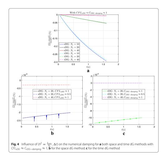
In conclusion, compared to the time dG method, the behavior of the space dG method across the physical interface is very interesting especially in cases involving a large number of physical interfaces. But future studies are necessary to understand and improve its behavior at external boundaries.
