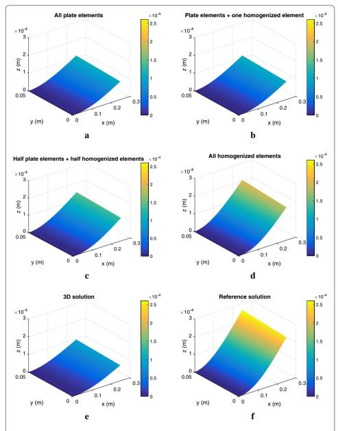
**Fig. 6** Displacement of the plate middle plane using plate theory (**a**), all plate theory elements except the homogenized (enriched) element (**b**), half plate theory elements (the triangles of the mesh in Fig. 2 with the right angle on the bottom) and half homogenized (enriched) elements (the triangles of the mesh in Fig. 2 with the right angle on the top) (**c**), all homogenized (enriched) elements (**d**), fully 3D FEM on a coarse mesh (**e**), fully 3D FEM on fine mesh (**f**)
