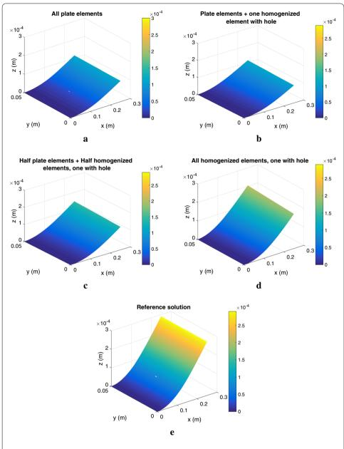
**Fig. 8** Displacement of the plate middle plane using plate theory (**a**), all plate theory elements except the homogenized (enriched) holed element (**b**), half plates theory elements (the triangles of the mesh in Fig. 2 with the right angle on the bottom) and half homogenized elements (the triangles of the mesh in Fig. 2 with the right angle on the top), one of them holed (**c**), all homogenized elements, one of them holed (**d**), fully 3D theory on the fine mesh (**e**)
