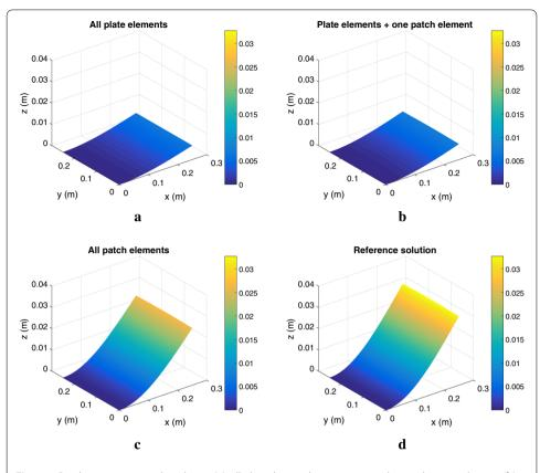
**Fig. 15** Displacement using plate theory (**a**), all plate theory elements except the patch super-element (**b**), all patches as depicted in Fig. 16 (**c**), fully 3D refined FEM (**d**)
