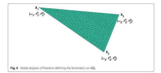
$$\begin{cases} u_{xy}^{e,1}(x,y) = \theta_1^x N_1(x,y) + \theta_2^x N_2(x,y) + \theta_3^x N_3(x,y) \\ v_{xy}^{e,1}(x,y) = \theta_1^y N_1(x,y) + \theta_2^y N_2(x,y) + \theta_3^y N_3(x,y) \\ w_{xy}^{e,1}(x,y) = \omega_1 N_1(x,y) + \omega_2 N_2(x,y) + \omega_3 N_3(x,y) \\ u_z^{e,1}(z) = -z \\ v_z^{e,1}(z) = -z \\ w_z^{e,1}(z) = 1 \end{cases}$$
