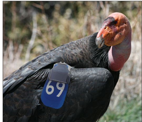
Fig. 1 Solar powered GSM-GPS geofence avian transmitter. Telemetry device is attached to the wing of a free-ranging California condor via patagial mount with an ID tag
