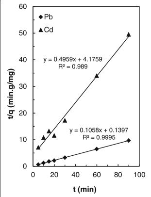
**Fig. 8** Pseudo-second order kinetic plot of Pb(II) and Cd(II) adsorption onto PANI/clay nanocomposite
