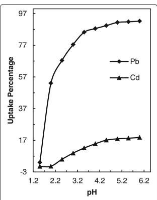
**Fig. 5** Pb(II) and Cd(II) ions removal with PANI/clay nanocomposite versus pH of solution
