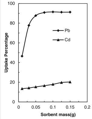
Fig. 7 Effect of adsorbent amount on Pb(II) and Cd(II) ions onto PANI/clay nanocomposite
