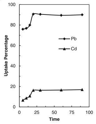
**Fig. 6** Dependency of contact time for adsorption studied ions onto PANI/clay nanocomposite
