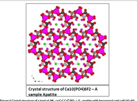
Figure 4 Crystal structure of a typical  $P6_3/mCa_4^l(PO_4)_6F_2$  apatite with hexagonal unit cell [43,44].
