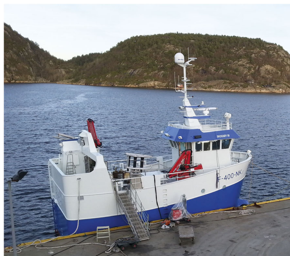
Fig. 3 Thor Arild built in 2015, length 14.97 m, width 6.6 m and 100 GT (with permission Skogsøy Båt 2016)
