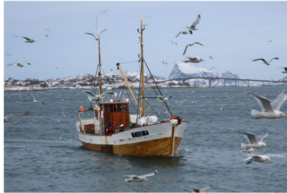
Fig. 2 Trålfisk built in 1962, length 15.48 m, width 4.75 m and 21 GT (with permission Fenstad 2017)
