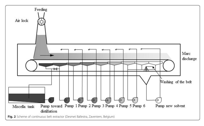
physical state allowing the pressure to remain close to atmospheric pressure [34]. Marc levels on the last three trays are controlled by chutes to ensure a defined throughput [35]. Direct steam is sparged in the DT by the bottom tray [35].
