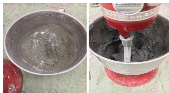
Fig. 3 Mixing of cement paste with SiO 2 materials
