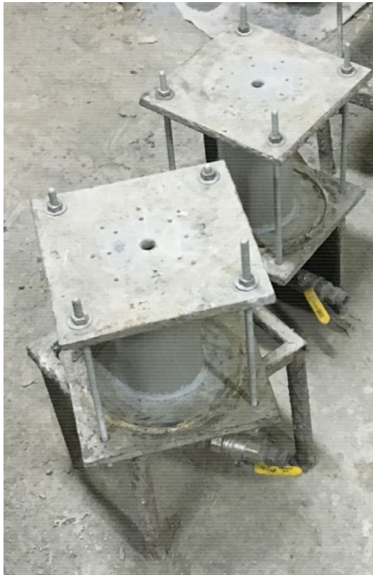
Fig. 9 PAC mold with preplaced ballast aggregates and their injection valve (ASTM C943, 2010)
