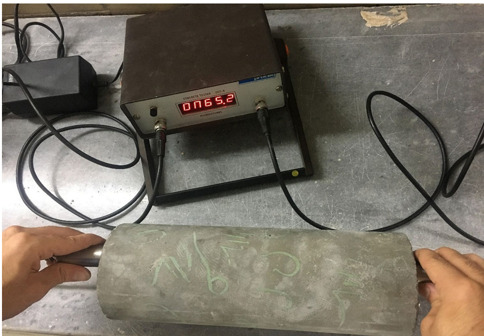
Fig. 5 Ultrasonic Pulse Velocity (UPV) test on PBAC specimens
