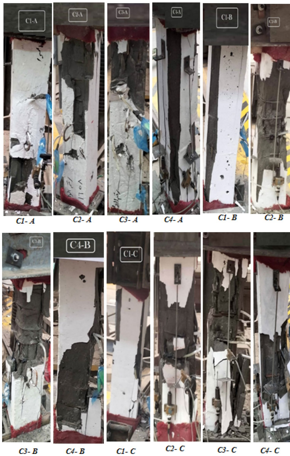
Fig. 7 Crack patterns for all column tested specimens
