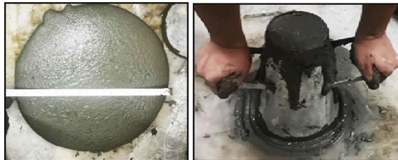
Fig. 1 Typical concrete slump flow test for UHPSSC mix
