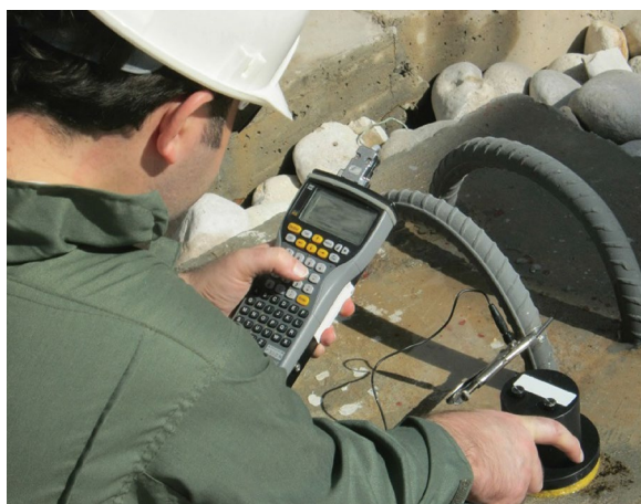
Fig. 3 The measurement of corrosion rate by galvanostatic pulse technique (Beirami & Ehteshamzadeh, 2016).
