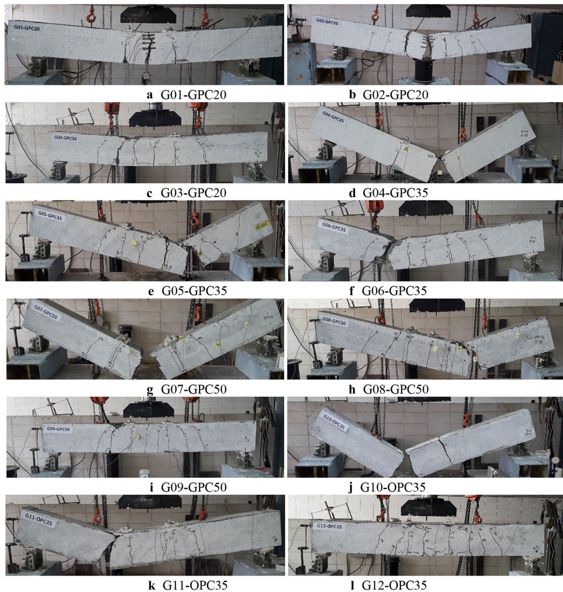
Fig. 6 Crack pattern and failure mode.
