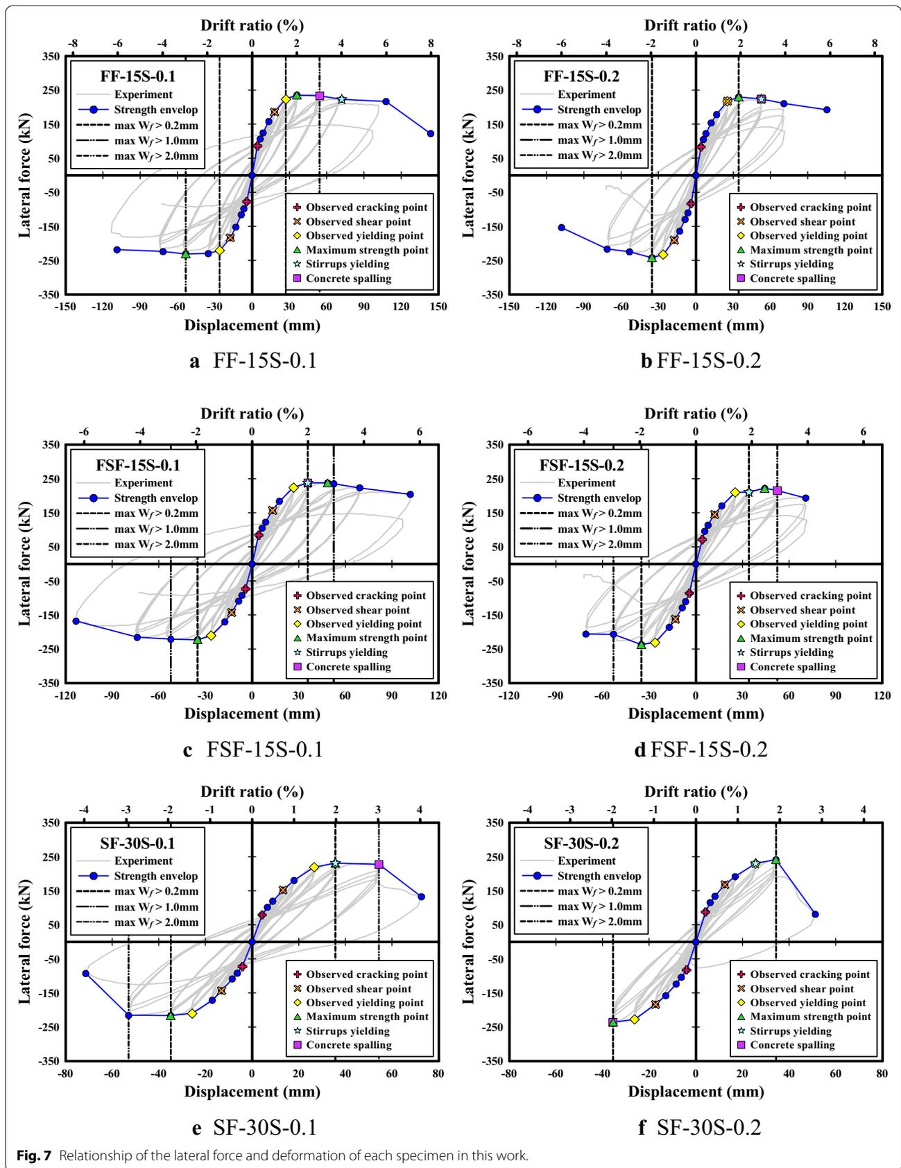
**Fig. 7** Relationship of the lateral force and deformation of each specimen in this work.
