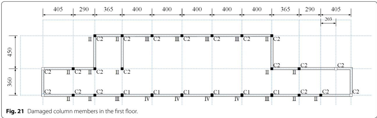
**Fig. 21** Damaged column members in the first floor.
