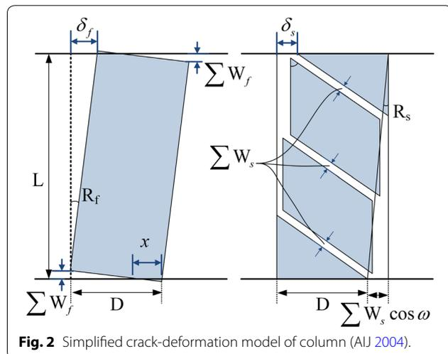
Fig. 2 Simplified crack-deformation model of column (AIJ 2004).
