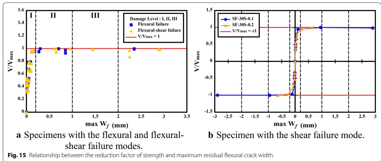
**Fig. 15** Relationship between the reduction factor of strength and maximum residual flexural crack width.
