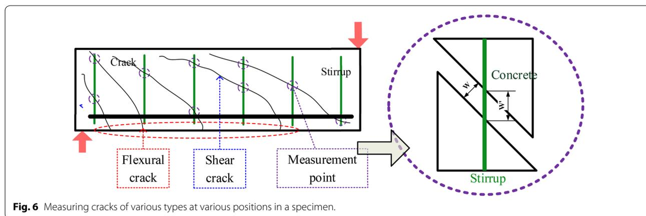
**Fig. 6** Measuring cracks of various types at various positions in a specimen.
