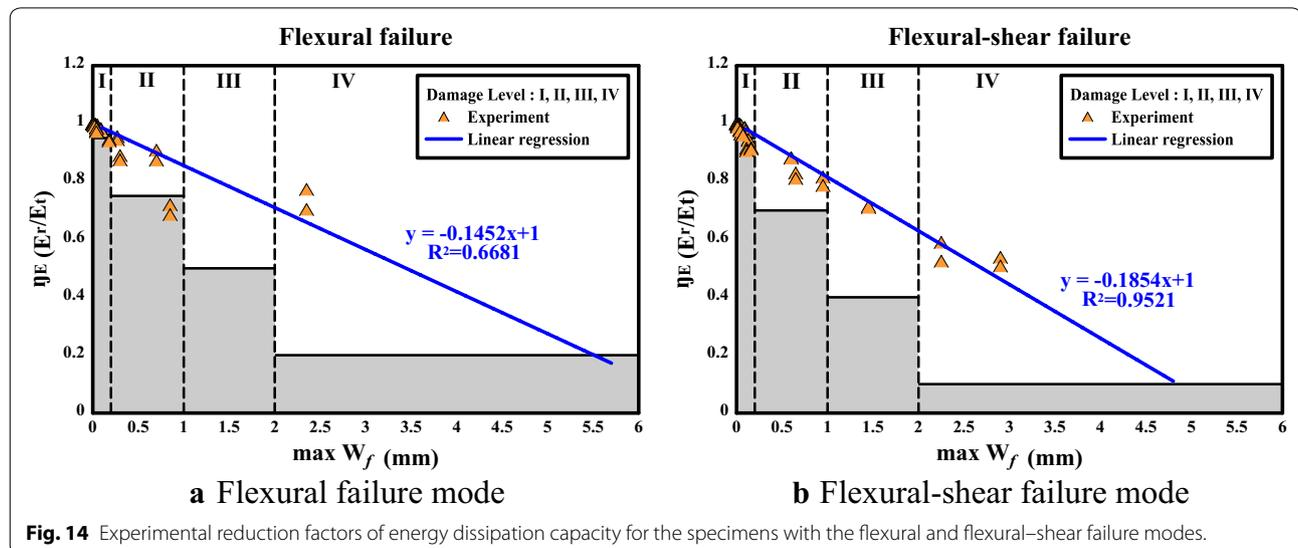
**Fig. 14** Experimental reduction factors of energy dissipation capacity for the specimens with the flexural and flexural–shear failure modes.
