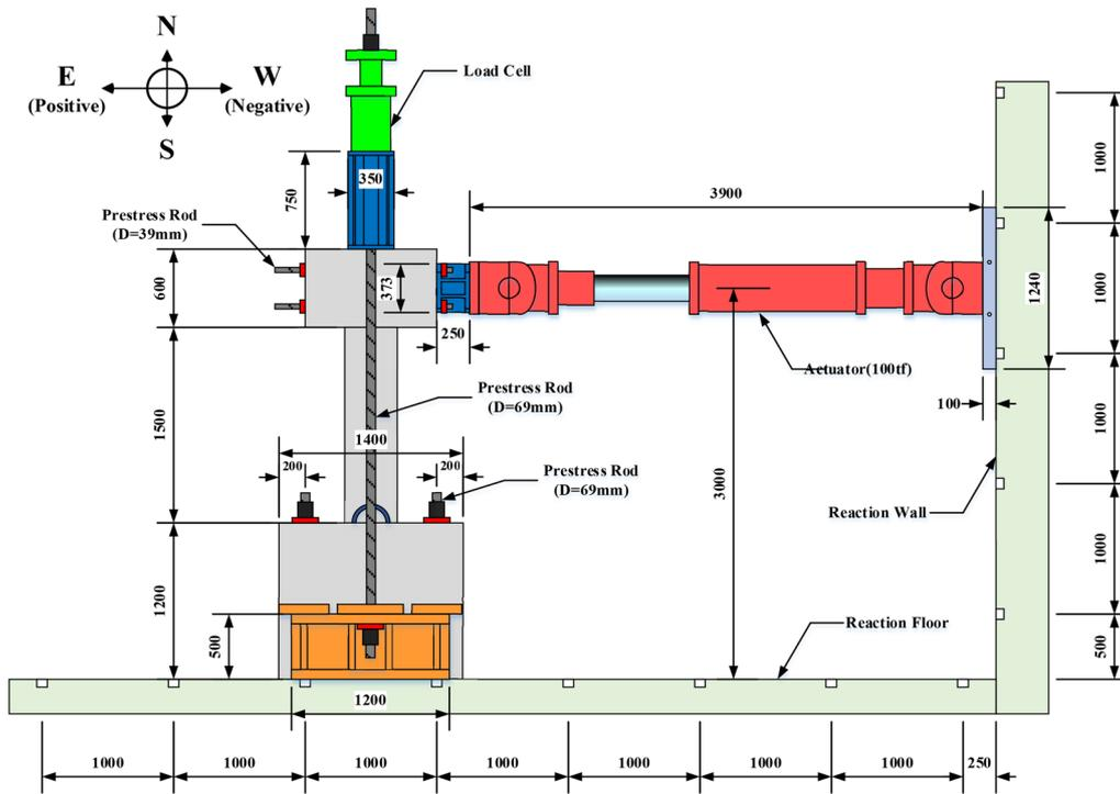
**Fig. 4** Applied loading system for the cantilever beam specimens in this work.
