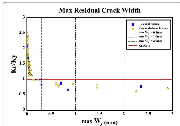
**Fig. 16** Relationship between the maximum residual flexural crack width and residual stiffness for the specimens with the flexural and flexural–shear failure modes.
