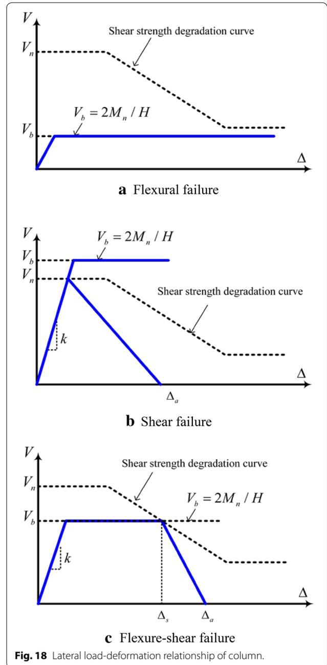
Fig. 18 Lateral load-deformation relationship of column.
