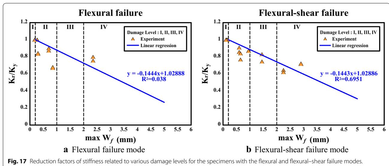
**Fig. 17** Reduction factors of stiffness related to various damage levels for the specimens with the flexural and flexural–shear failure modes.
