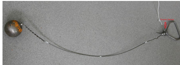
Fig. 4 The prototype of biomechanical feedback device for hammer throw training
