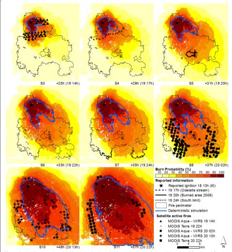
**Fig. 7** Probabilistic predictions (*shaded colours*) and deterministic simulations (*blue line*) of fire spread for the Tavira wildfire— $t_0$ . Simulations initialized at the reported ignition point (start: day 18 at 13 h; durations: 25 (S3), 28 (S4), 31 (S5), 33 (S6), 35 (S7), 37 (S8), 48 (S10) and 57 (S11) hours, respectively) and fire front location at the specified hour (time step), obtained from both satellite and reported information
