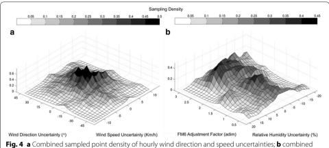
**Fig. 4** a Combined sampled point density of hourly wind direction and speed uncertainties; **b** combined sampled point density of daily relative humidity uncertainty and ROS adjustment factor for fuel model 6
