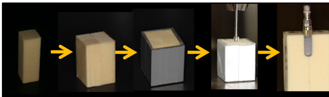
Fig. 1 Flow of a divided block specimen. Four divided block specimen was assembled by tape. Their circumference was fixed with metal jigs and the implant was inserted according to the manufacturer instructions. After the placement, the metal jigs and two of the divided block were removed carefully
