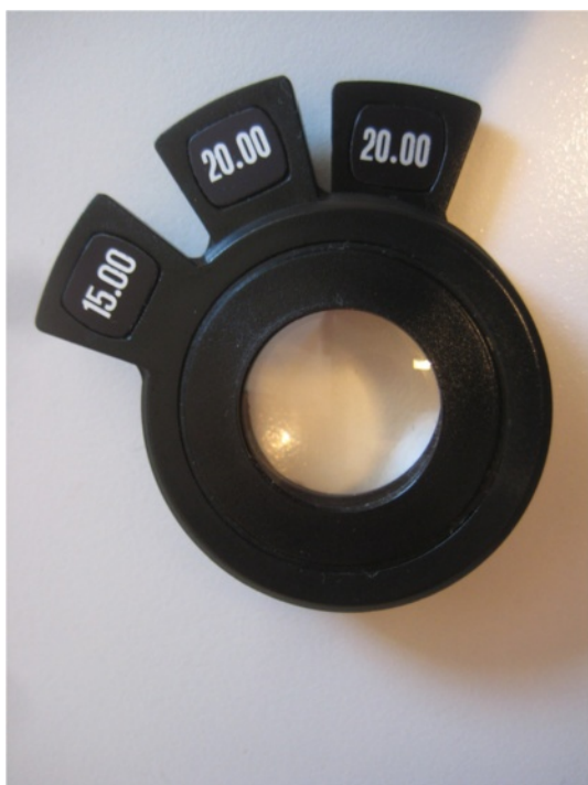
Figure 4 “Lens sandwich” of altogether +55D power (+20/+20/+15D from lens trial set). The quality of this “lens sandwich” suffices for adequate diagnosis of the disease condition despite its obvious suboptimal optical properties (in comparison to a single aspheric lens made from glass) - see also Figure 3 (+55D is the power of the original el Bayadi lens (El Bayadi 1953)).
