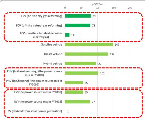
**Fig. 1** Comparison of CO<sub>2</sub> emissions (well-to-wheels JC08 mode). *Source*: "Report on overall efficiency and GHG emissions by type of vehicles," Japan Automobile Research Institute, March, 2011. "The roadmap of the hydrogen and fuel cell strategy, Revised," Hydrogen and fuel cell council, METI, March, 2016. *Note* The CO<sub>2</sub> emission of EV (the power source mix in FY2012) is estimated suitable to the power source mix in FY2012 by the Hydrogen and fuel cell council, METI
