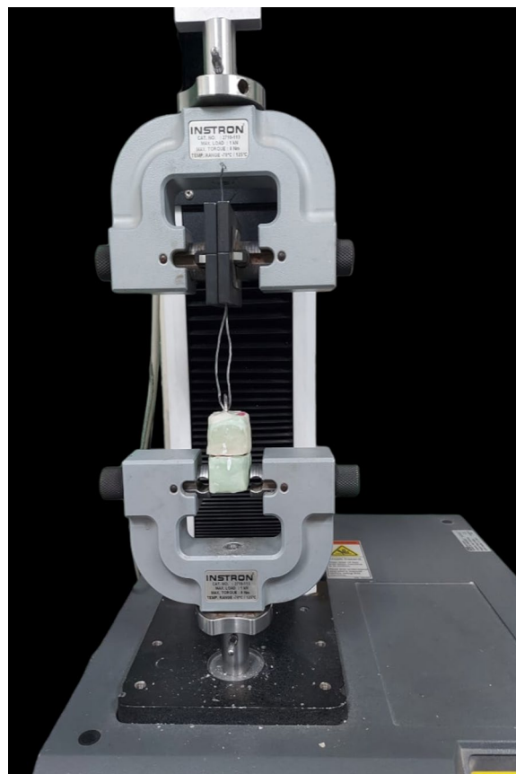
Fig. 4 Two resin blocks, one with the ball abutment and the top one with the tested attachments attached to the Instron universal testing machine for measuring retention values
