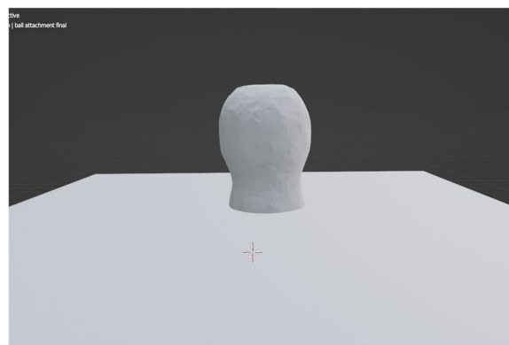
Fig. 1 STL file acquired by an optical scanner and representing the ball abutment geometry which is composed of the ball abutment head and ball surface undercut
