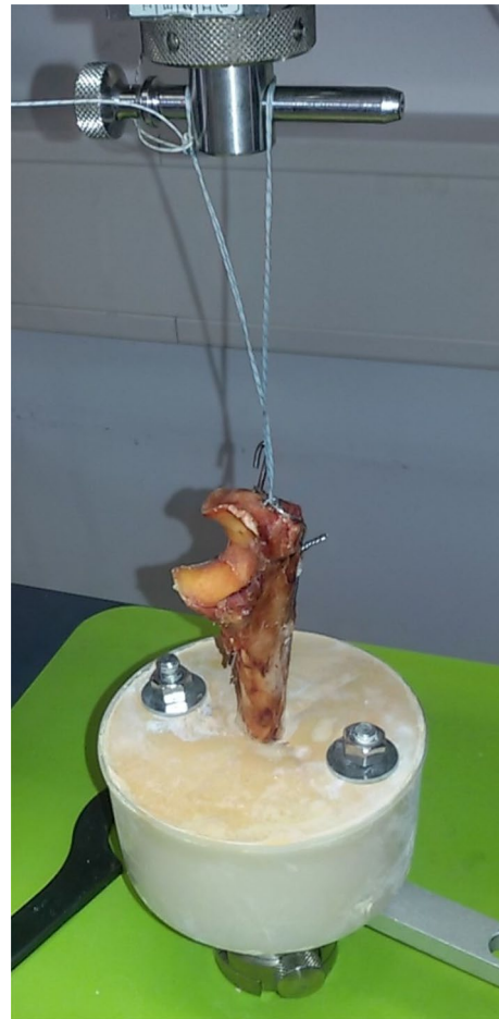
Fig. 4 Test setup with the TBW of the proximal ulna under the uniaxial tension testing system (Zwick/Roell®) while fixing the tricortical k-wire with a highly cross-linked 2-mm FiberTape®
