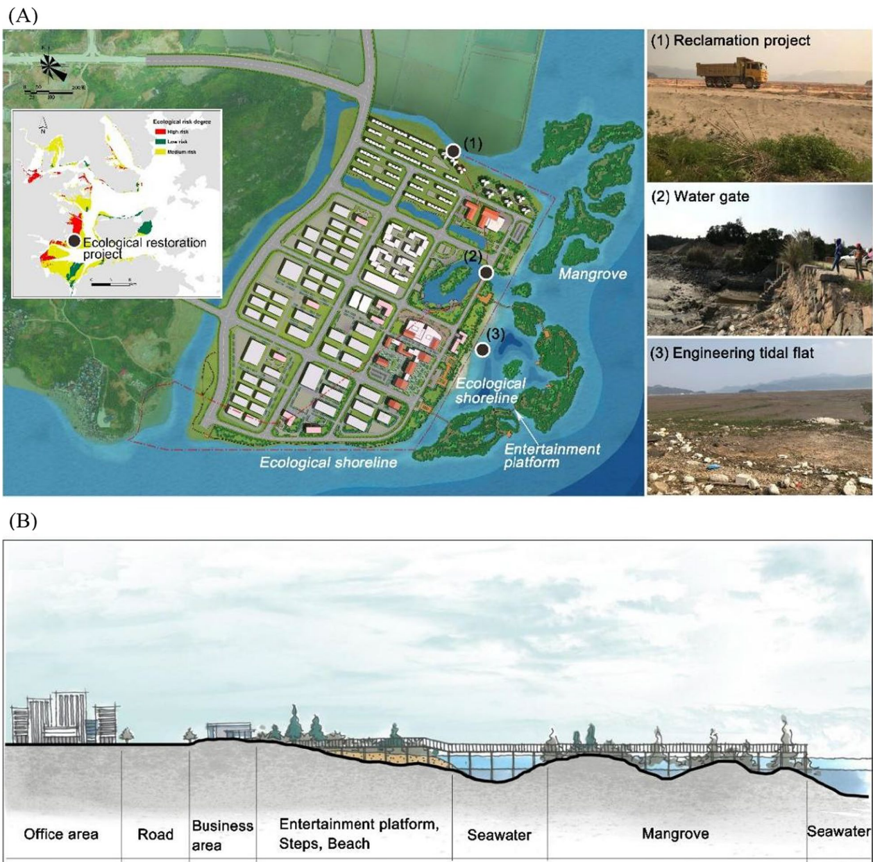
Fig. 6 A Ecological restoration project design. B Cross-section of the ecological restoration project on the western coast of Sansha Bay
