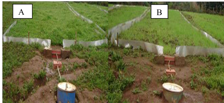
Fig. 3 Experimental setup of runoff plots with runoff collection tanks. a Grazing land and b cultivated land
