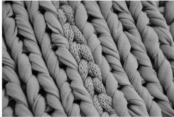
Fig. 1 Knitted textile with an integrated knitted sensor (in the middle)
