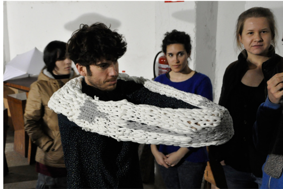
Fig. 8 Sound Embracers (v.2) is made of a knitted net, stretch sensors, and speakers. It relates to the body by constraining the arms. Its context of use is music performance
