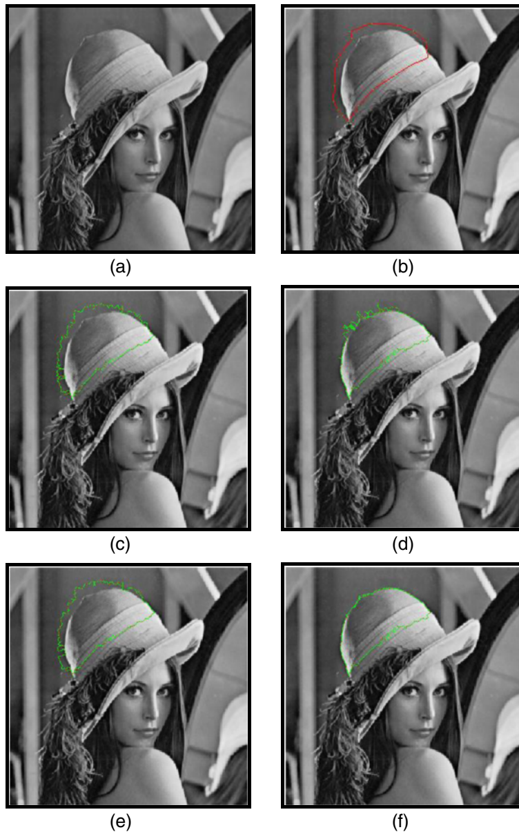
Fig. 4 Performance of the proposed method on Lena image compared to the DWT based method with the strong objects. (a) Lena original image (b) Selected Lena hat. (c) With DWT method at 400 iterations (d) With DCWT method at 400 iterations (e) With DWTB method at 400 iterations (f) With proposed method at 400 iterations
