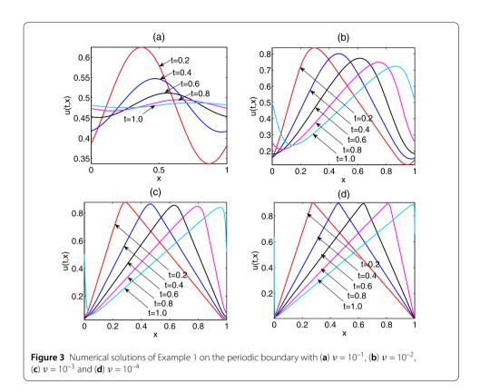
$10^{-4}$ . In other words, as  $\nu$  becomes smaller, the curves steepen and develop a shock-like discontinuity. As seen in Fig. 3(c) and (d), the proposed method is able to capture the sharp front very well under the periodic boundary conditions. Note that this test is valuable, since the Burgers equation has been studied in a limited work over the periodic boundary conditions compared to non-periodic boundary conditions.
