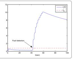
and according to (83) and (84), the residual evaluation function  $J_r(t)$  in Figure 5 indicates that the fault is detected at approximately t = 42.44 s.
