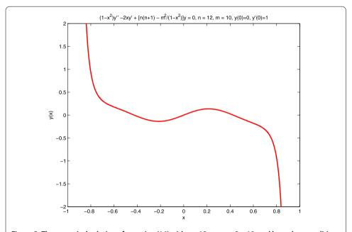
Figure 5 The numerical solution of equation (14) with n = 12, m = n - 2 = 10, and boundary conditions y(0) = 0 and y'(0) = 1. The solution is nonoscillatory as two extrema of the same kind do not appear in the interval (-0.60, +0.60) that is determined from equation (19).
