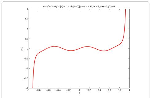
Figure 4 The numerical solution of equation (14) with n=12, m=8, and boundary conditions y(0)=0 and y'(0)=1. The oscillations terminate at  $x_*\approx \pm 0.77$ , as predicted by equation (19).
