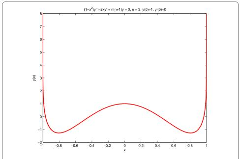
Figure 1 The numerical solution of equation (5) with n=3 and boundary conditions y(0)=1 and y'(0)=0.
