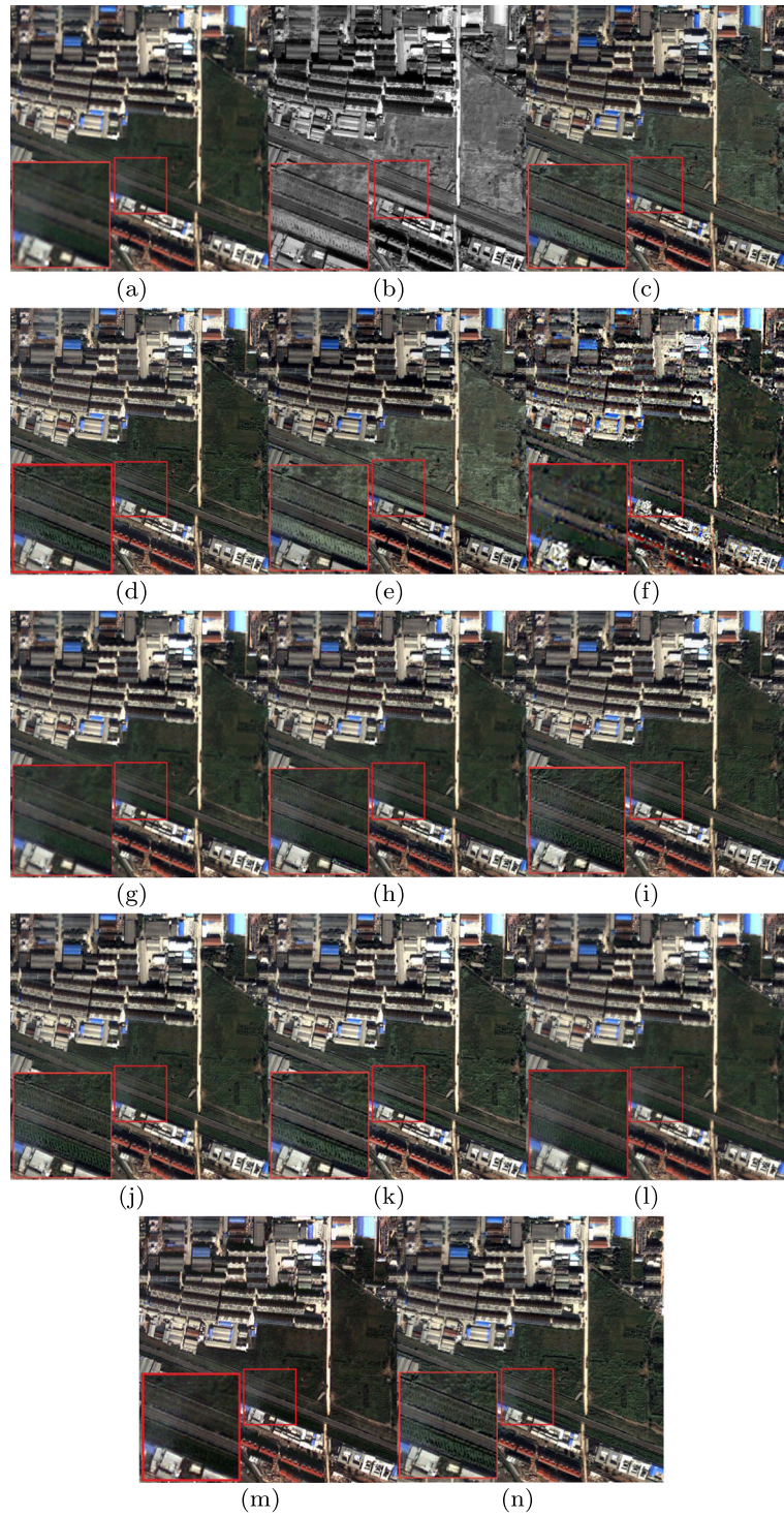
Fig. 10 Fusion results of the real QuickBird-2 dataset. a Upsampled MS image ( 1024 \times 1024 ). b PAN image ( 1024 \times 1024 ). c IHS method. d AIHS method. e PCA method. f BDSD method. g PRACS method. h SFIM method. i Indusion method. j MTF-GLP method. k CAE method. l MSGF method. m PNN method. n Proposed method
