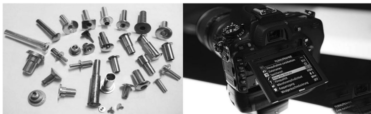
Fig. 1 Precision rivets of different sizes for experiments and photo acquisition equipment
