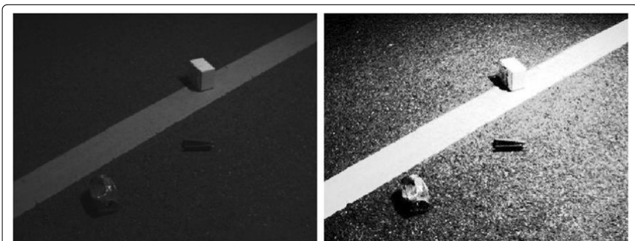
Fig. 5 Comparison of histogram equalization image enhancement effects. a Image before histogram equalization processing. b Image after histogram equalization processing
