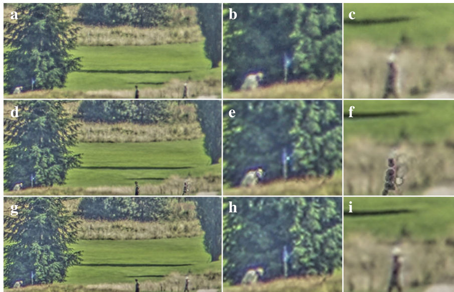
Fig. 7 Turbulence mitigation on a golf course scene. The top row shows a still from the raw video (a) and two cut-outs around the hole (b) and a walking golf player (c). The middle row shows the processing results with the global turbulence mitigation method and the bottom row shows the result for dynamic turbulence mitigation with TV-L1 optical flow. The walking golf player is about 25 \times 70 pixels in size
