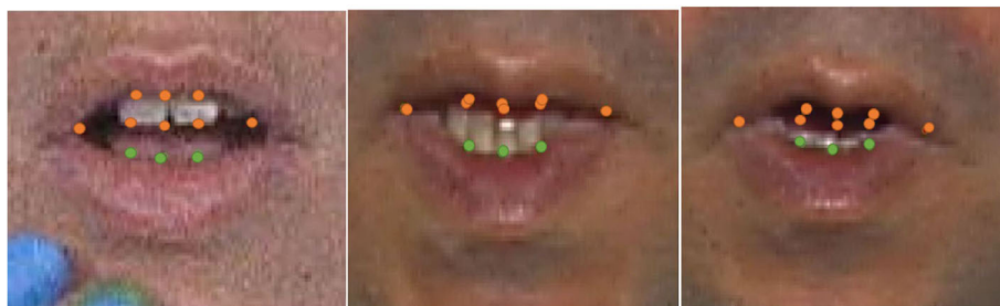
Fig. 14 Examples showing initial mistaken CLNF landmarks (orange points) and corrected landmarks using the proposed method (green points) for the inner lower lip
