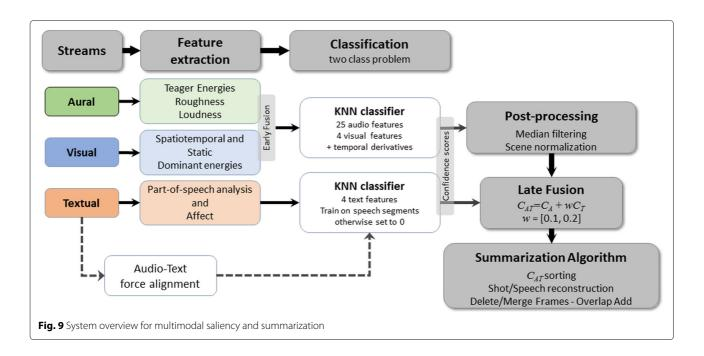
application of the energy operator is preceded by bandpass filtering, using 25 linearly-spaced Gabor filters with 50% overlap, resulting in mean instantaneous energies derived from each filter.
