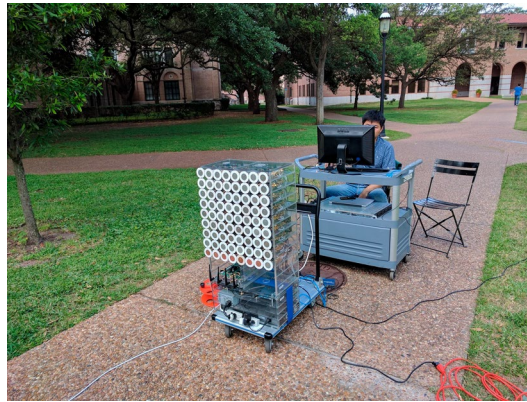
Fig. 2 Channel measurements setup with large-array base-station. The plot comes from [26]
