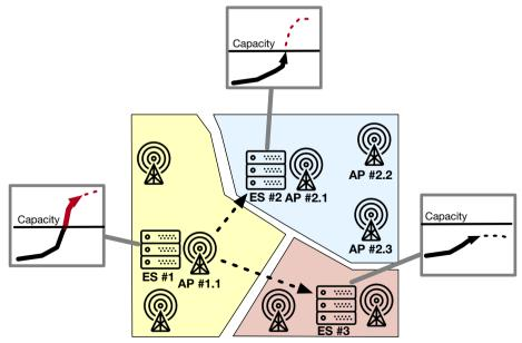
Fig. 1 Reallocation of workload. ES 1 is over capacity, so AP 1.1 may decide to reallocate new workload from its users to ES 2, the nearest ES (proximity strategy), ES 3, with the lowest workload (bottom-up strategy), or offload the workload to cloud (cloud strategy). (Figure originally in [10].)
