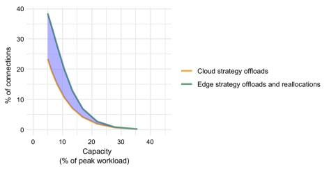
**Fig. 5** Superfluous reallocations. The difference (blue area) between the number of offloads for cloud strategy (orange line) and the number of reallocations and offloads for an edge strategy (green line) is the number of superfluous reallocations, shown here as a proportion of all connections. (Figure originally in [10].)
