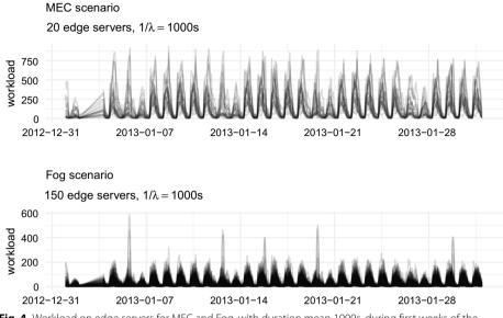
Fig. 4 Workload on edge servers for MEC and Fog, with duration mean 1000s, during first weeks of the observation period 2013–2014. A service break is clearly visible in the first week
