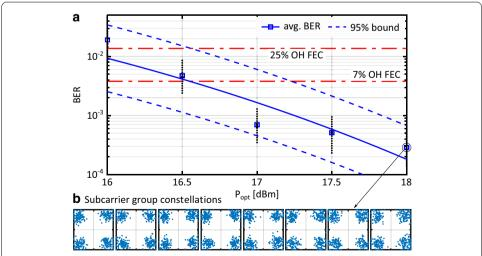
**Fig. 7** Transmission perfromance measurement results for the experimental real-time ARoF fronthaul demonstration: **a** real-time BER in dependence of optical power after two-tone generation and associated statistics, **b** observed constellations for the 800 MHz wide 5G NR OFDM signal. BER: bit error rate, OH: overhead, FEC: forward error correction
