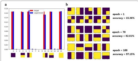
**Fig. 9**  $2 \times 2$  Bars-and-Stripes samples generated from QCGAN. **a** The final probability distribution of the generative BAS data. **b** BAS samples generated from QCGAN with different epoch (For illustrative purpose, we only show 10 samples for each situation)
