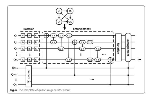
generator is realized by a PQC based on quantum gate computing mechanism, which is composed of rotation layers and entanglement layers alternately arranged. Due to the unitary nature of the quantum gate set, if the rotation layer and the entanglement layer alternately perform operations and form a sufficiently long layer sequence, any unitary transformation can be performed on the initial state in theory.
