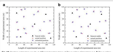
**Fig. 10** Position estimation results at different iteration times. **a** The number of iterations is 1. **b** The number of iterations is 4
