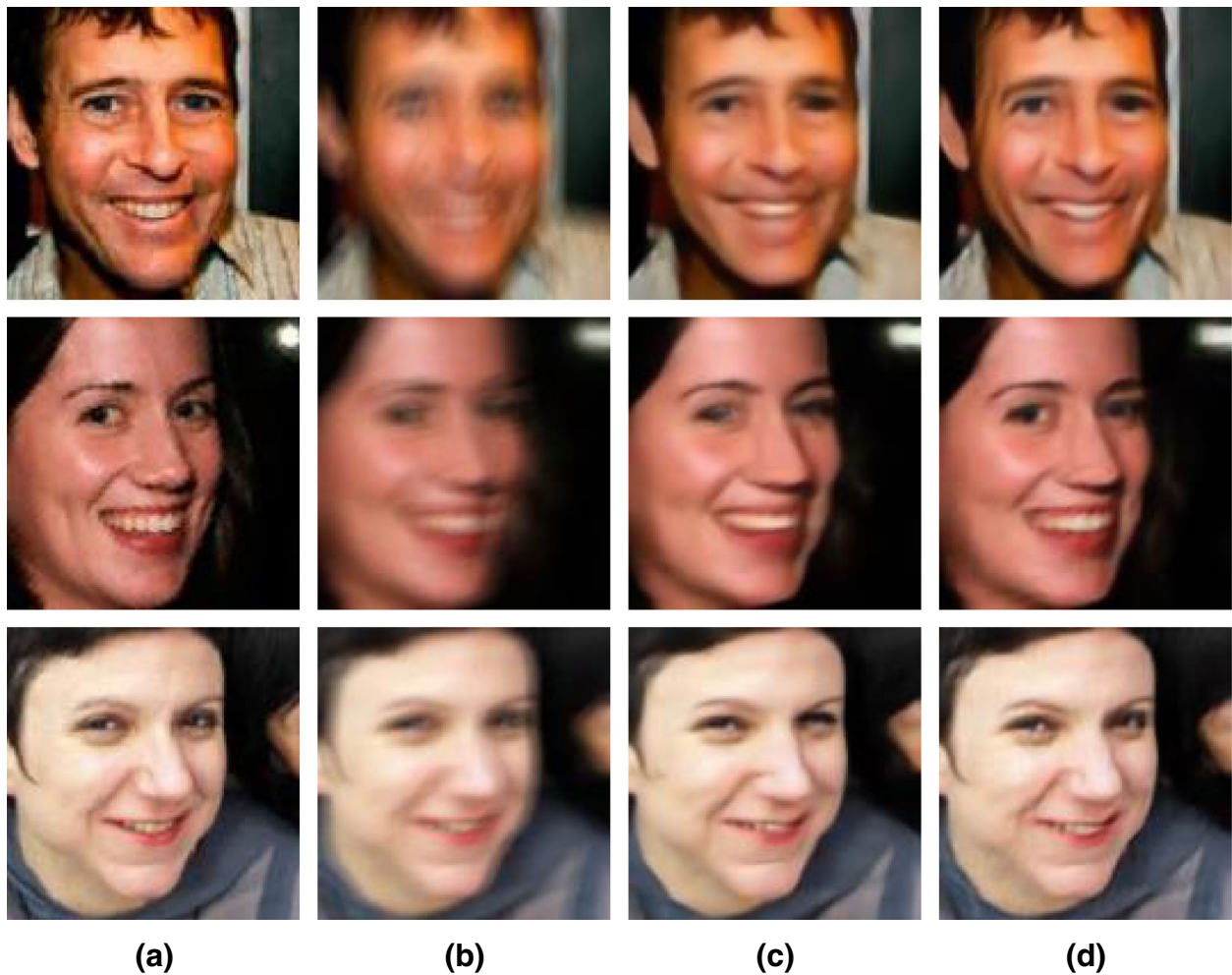
Fig. 4 Ablative study for transfer learning model. a Ground truth images. b Blurred images. c Deblurred results via a single-task model. d Deblurred result via a multi-task model
