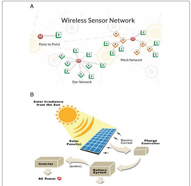
**Fig. 1** Photovoltaic cell and system. **a** Wireless sensor networks system. **b** Explanation of the principle of solar cell power generation system: sunlight is irradiated to the solar panel to generate electric current, which is provided to the electric equipment or battery energy storage system
