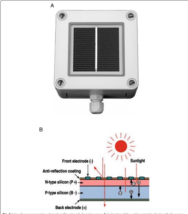
**Fig. 2** Solar cell power generation schematic. **a** The solar cell of wireless sensor. **b** Explanation of the working principle of solar cells: the n-type silicon's spare electrons jump over to fill the gaps in the p-type silicon. The n-type silicon becomes positively charged, and the p-type silicon is negatively charged, creating a current field across the cell
