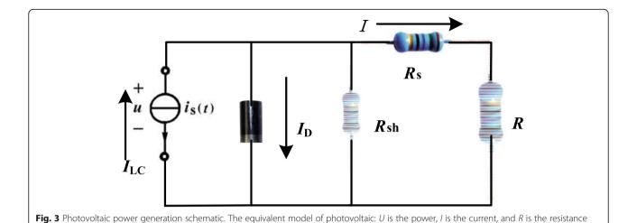
the constant current source, and the R is the series resistance of the multi solar panel, which can be obtained according to Kirchhoff's current law:
