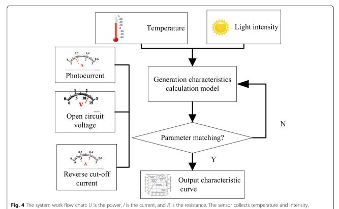
calculates the parameters of the equivalent model, and outputs the results after matching the parameters
