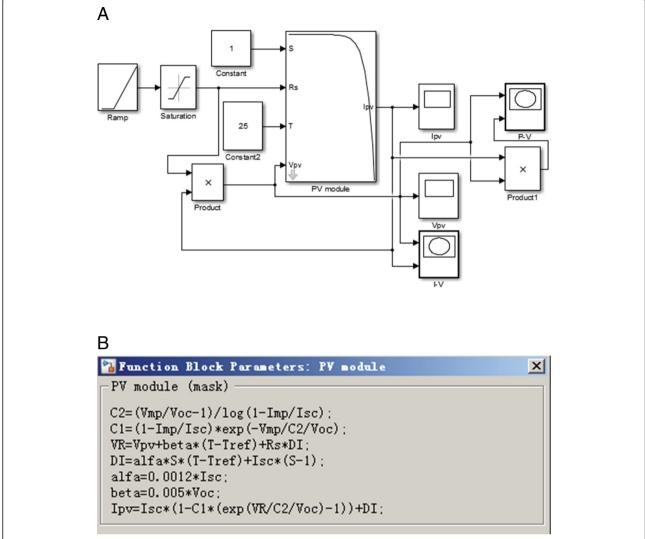
Fig. 5 MATLAB simulation block diagram and parameter setting. a The simulation block diagram of solar cells in MATLAB software: ramp and so on are input signals, The PV model is a mathematical model described in the chapter 2.2. I–V, and P–V are the oscilloscopes used to display the results. b Parameter setting of simulation block
