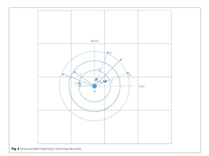
Within this subset, the location  $L_i(f_i)$  of every fingerprint  $f_i$  locates in the constrained area *ABCD*.
