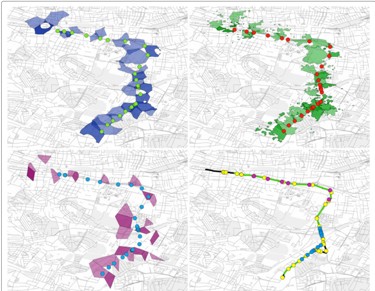
Fig. 9 Trajectory 4. Estimation of event positions based on different coverage prediction methods: Coverage prediction ( top left ), coverage prediction including height and building model ( top right ) and Voronoi tessellation ( bottom left ). The last picture shows the original trajectory recorded using a GPS tracker ( black ) and the estimated trajectory based on event positions derived from the top right image ( green ). The purple points indicate an active speech session, the blue ones a data session, respectively. The yellow points are the actual event positions which have been recorded using a handset
