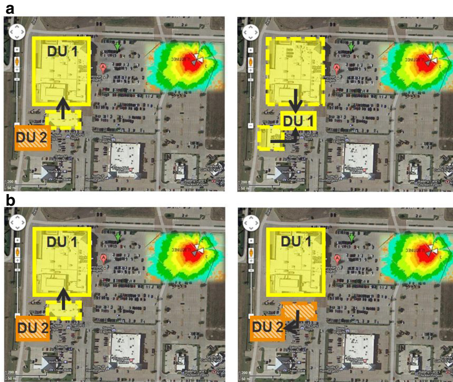
Fig. 8 Reclustering cases: a relocation of a DU; b reassignment of a building to a new DU
